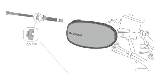
If necessary, use the 7.5mm bush to move the handguard further away from the handlebars.
